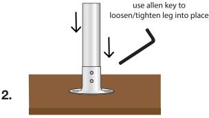
**2.** Insert an upright leg into the Bottom Bracket. You may need to loosen the allen screws in the Bottom Bracket to allow the leg to pass through. Once the leg is in place tighten the allen screws.
