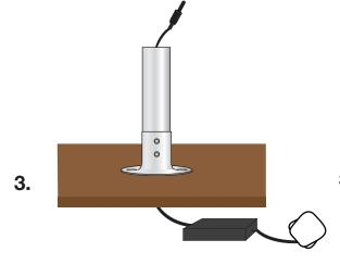
3. Thread the transformer cable up one of the legs.
